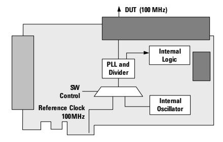
The clock is generated using the system-provided 100 MHz PCI Express reference clock. However, there is also the possibility to use the internal clock oscillator if for some reason the system clock cannot be used. The reference clock and the internal clock are used for the internal logic of the PTC as well as for providing the clock to the DUT plugged onto the PTC.
