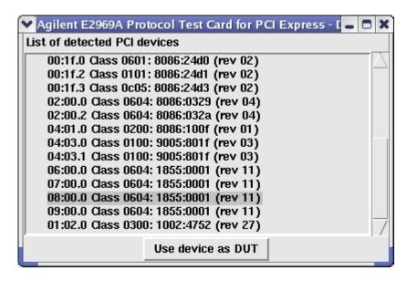
3 From the list of detected PCI Express devices, select your DUT and click the *Use device as DUT* button.
