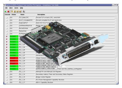
The PTC performs tests to verify and ensure compliance with PCI Express as defined by the PCI-SIG.
